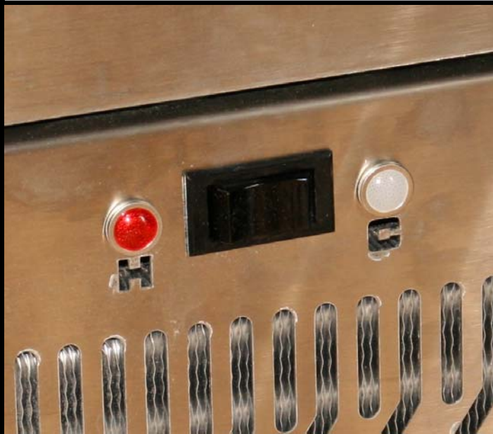
Illustration 2.A- Dual Serving Module On/Off/Mode Switch
